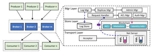
Fig. 3. The overview of BPS architecture.
