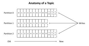
Fig. 4. The process of appending messages to partition.
