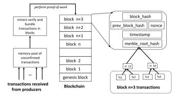
Fig. 2. The generic architecture of blockchain platform.
