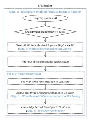
Fig. 5. The overall relationship between Algo. 1, 2, 3, and 4 employed by BPS.
