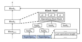
Fig. 6. Traceable topic operation in blockchain.
